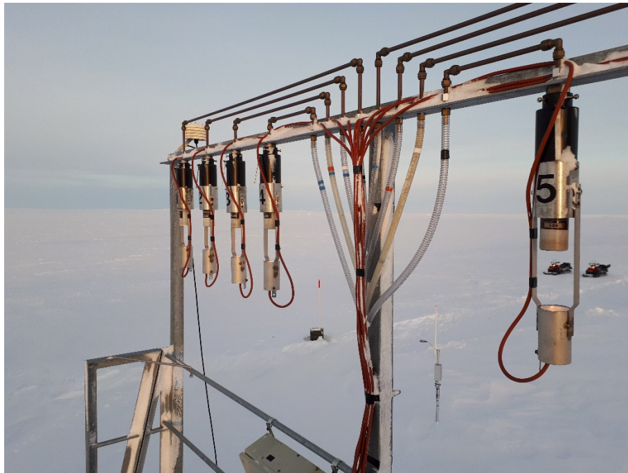
Figure 4.2. Sampling inlet for the filter pack sampler on the roof of the Air Observatory. Photo: Jakob Boyd Pernov.
