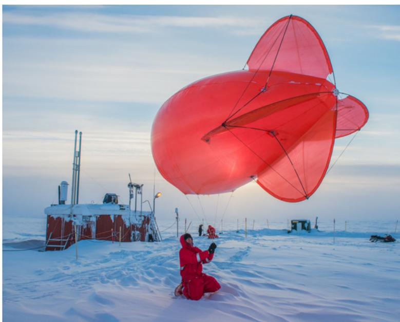
Figure 4.1. The 9 m<sup>3</sup>-tethered balloon in front of Flyer's Hut ready to go. Photo by courtesy of Esther Horvath, Alfred Wegener Institute, Helmholtz Centre for Polar and Marine Research.
