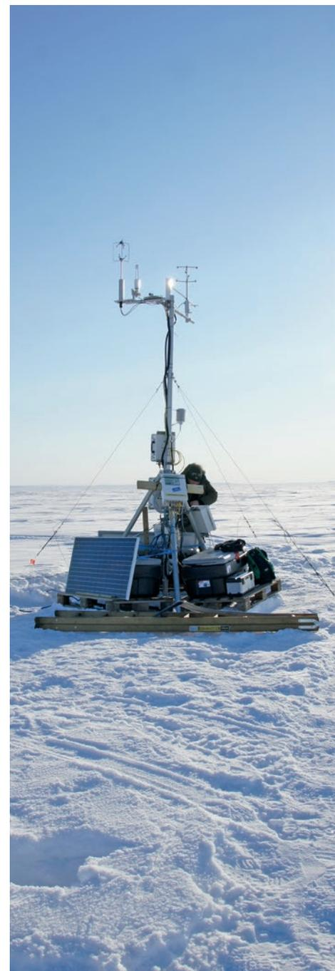
Flux system for measuring fluxes of carbon dioxide and methane.
