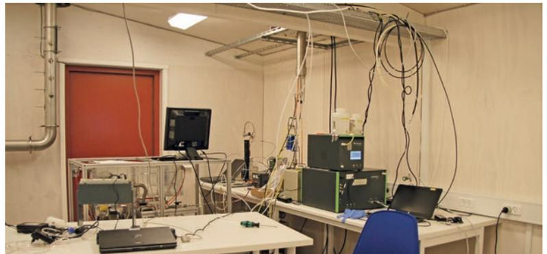
Chemical Ionization - Atmospheric Pressure Interface - Time-of-Flight mass spectrometer (CI-API-TOF).
