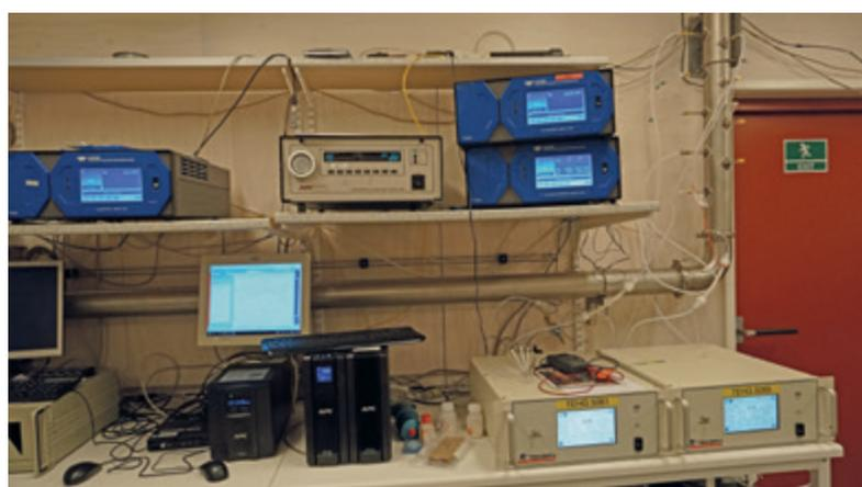
Figure 1.1. The instruments for mercury measurements in action in the air-monitoring house.
