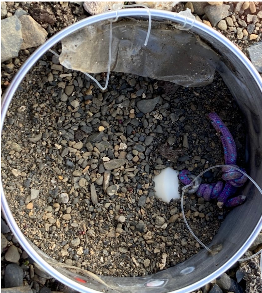
Figure 5.4. We buried plastic pieces in field pots close to the Villum Research Station for one year and then isolated microbial strains from the plastisphere in the laboratory.
